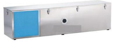
The UV FAN is an air purification device consisting of a structure in extruded aluminum, coated by epoxy powder. **Front/Side pre filter** allow air to enter and exit from other ends. An internal fan blower conveys air from the external room to the inside of the germicidal box to be purified from air borne contaminants.
