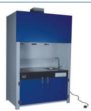
Fume Hood are designed to contain and exhaust toxic, obnoxious, pungent smelling gasses to protect personnel and equipment in the laboratories. The fume hood comprise with international standard on fume handling systems. A motor driven dynamically balanced blower with minimal vibration and noise level creates negative pressure and sucks contaminated air from work area and throws the same in high-up atmosphere through ducting's.
